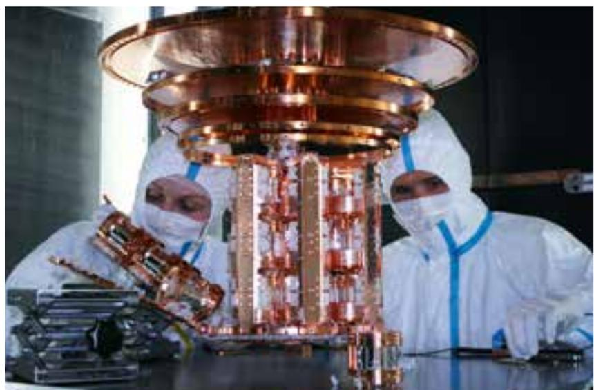
Detector mounting at Gran Sasso for the CRESST direct detection experiment. At CRESST searches for dark matter particles scattering on nuclei are conducted at very low temperatures. If such a scattering occurs, the minute amount of heat produced in the collision can be detected.
